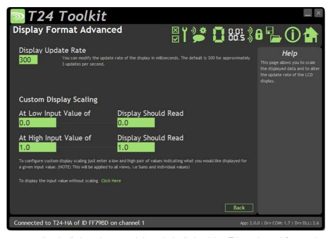
Here you can adjust the display update rate and also scale the displayed data. This may be used, for example, to convert the data from a WIRELESS-T24-SA calibrated in kg so that the handheld display shows lb.
