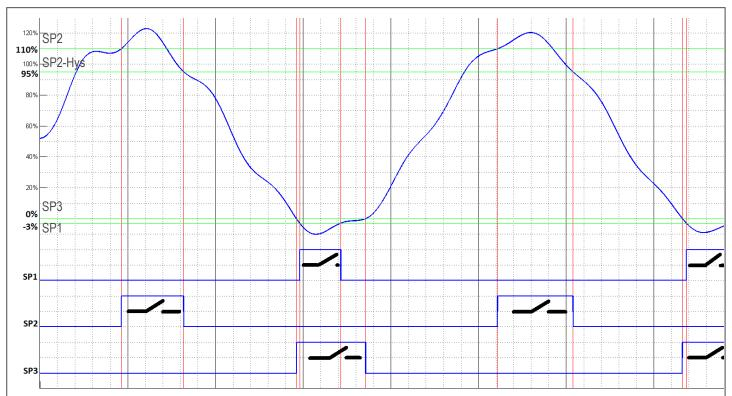
Enter menu "6 –SPt" (SENSY access code = 7) and configure the parameters as shown in the table below.
