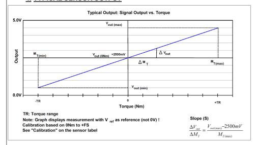
Vout(max) and Vout(min) are defined by the slope of each sensor. This means that the output signal may vary between 0.5V and 4.5V; the actual signal output range depends on the calibration value and the torque range.
